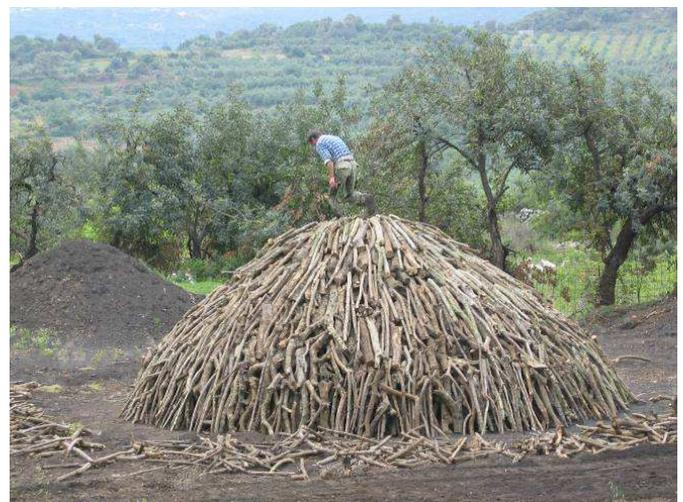
The basic structure of the pile requires "many hands working" and effort (**picture left**). The "pole wood building" (before the final "roof") is more a work for a specialist with experience (**picture right**).
